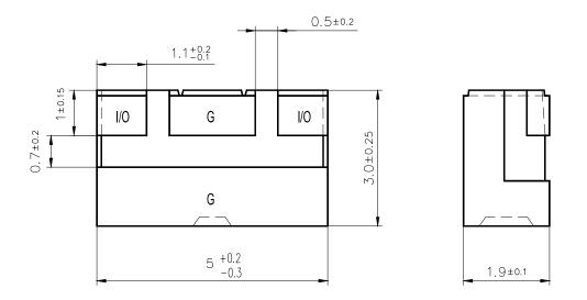
View from below onto the solder terminals and view from beside Marking: 'EPCOS Logo' on top of the filter
