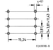
Hole arrangement View in mounting direction
