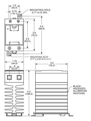
Recommended Torque Range for Terminal Screws: Control: 5 - 6 in lb (0.6 - 0.7 Nm). Output: 10 - 15 in lb (1.1 - 1.7 Nm).
