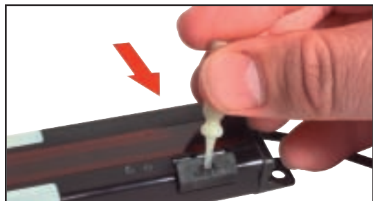
Figure 7. PVA cover removal
