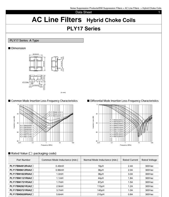
Operating Temperature Range (Ambient Temperature Range + Winding Temperature Rise): -25°C to 120°C Winding Temperature Rise (at Rated Current) (max.): 60K
