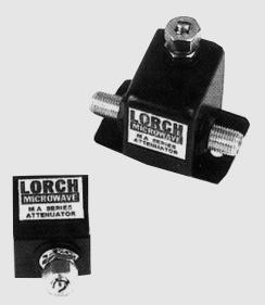
orch Microwave's MA-Series, Manual Attenuators, are miniature components which may be adjusted manually by mechanical rotation to provide a useful range of smoothly variable attenuation over the frequency range DC to 400 MHz, with low VSWR and low minimum insertion loss.
