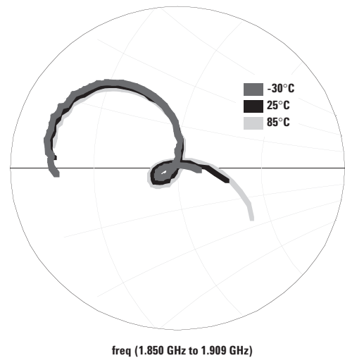
Figure 7. Tx port impedance (8 dB circle).
