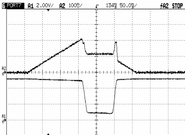
2009B SOT 502 #1 - Current ramp (5V) R adj =249ohms, R fault =499ohms A1: Vout (2V/div) A2: Iout (500mA/div)
