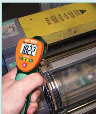
Electrical Troubleshooting for hot spot detection
