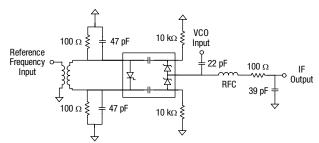
Input transformer: 10:1 step down impedance ratio.
