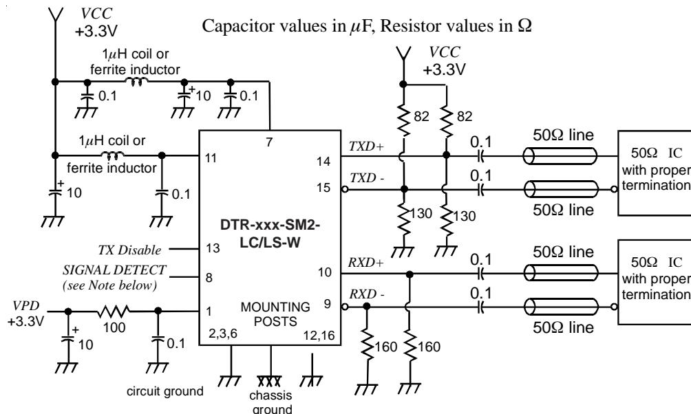
Note: If signal detect is LV-PECL, a termination resistor of  $160\Omega$  to GND is required
