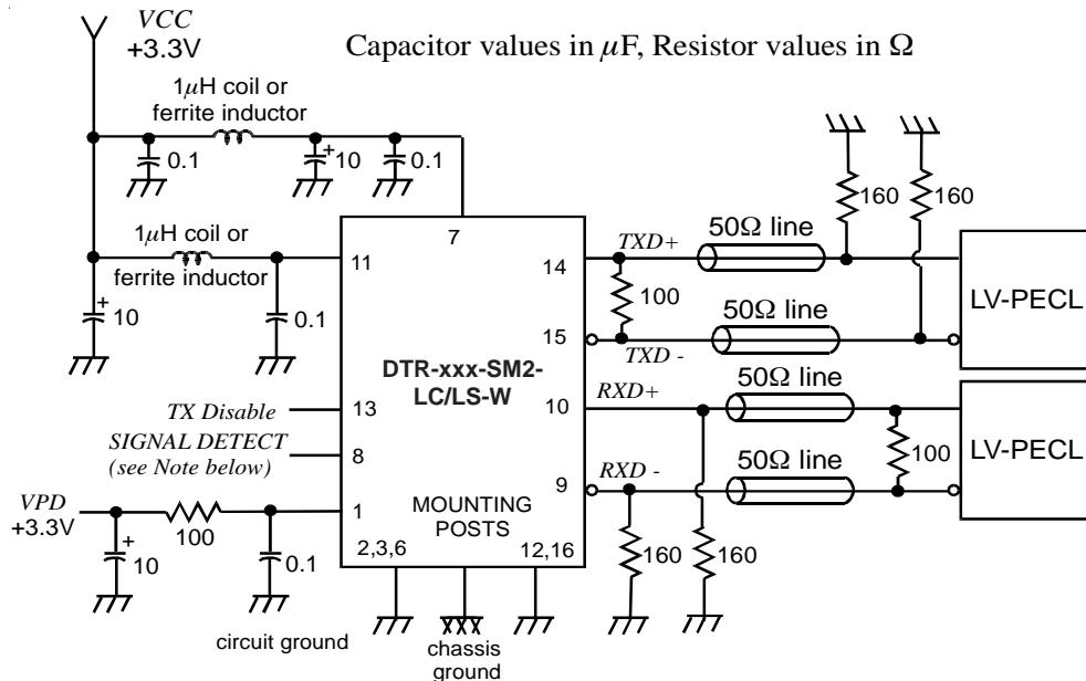
Note: If signal detect is LV-PECL, a termination resistor of  $160\Omega$  to GND is required
