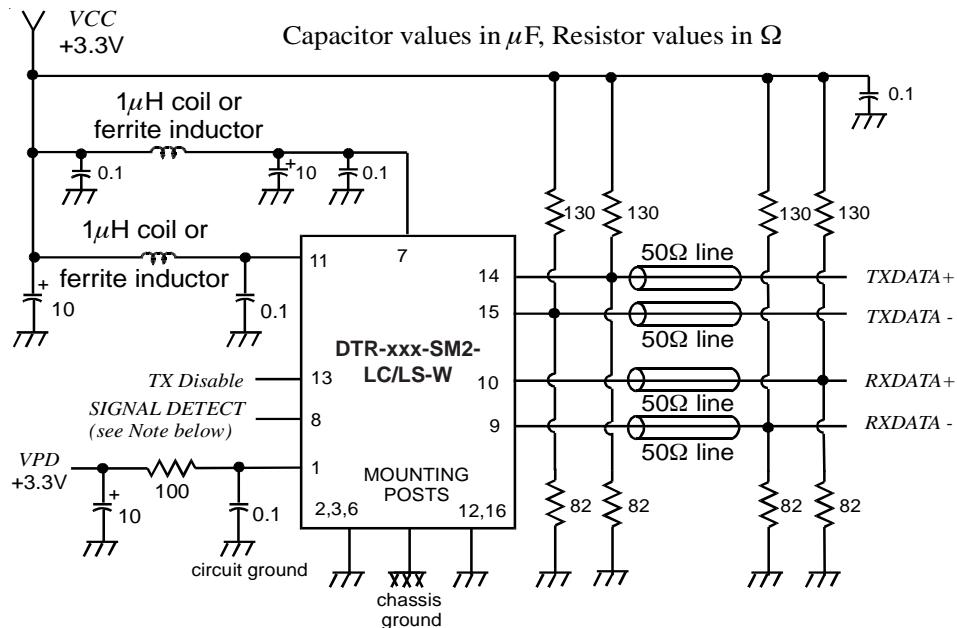
Note: If signal detect is LV-PECL, a termination resistor of  $160\Omega$  to GND is required.
