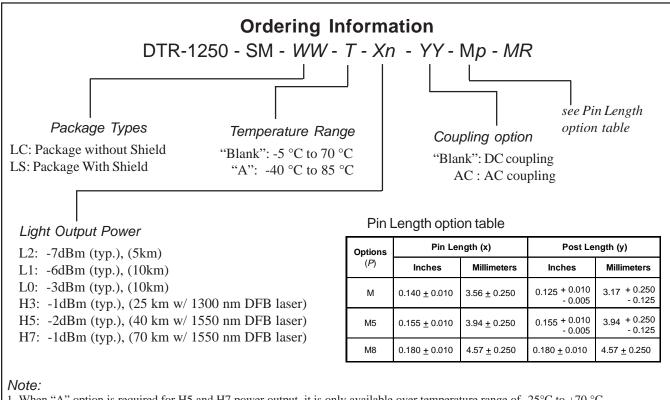
When "A" option is required for H5 and H7 power output, it is only available over temperature range of -25°C to +70 °C.
