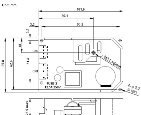
AC Input Connector (CN1): Molex 5277-02 or equivalent
