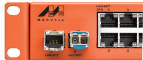
Auto-Media detect UpLink for copper or fiber
