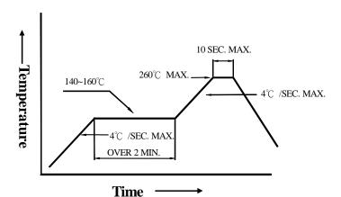
3. DIP soldering (Wave Soldering) :
