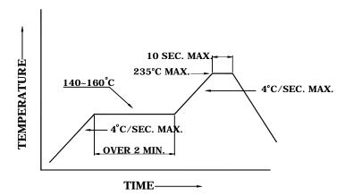
DIP soldering (Wave Soldering)
