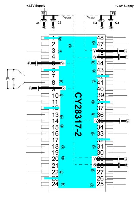
FB = Dale ILB1206 - 300 (300 $\Omega$  @ 100 MHz) or TDK ACB2012L-120 Ceramic Caps C3 = 10–22  $\mu$ F C4 = 0.005  $\mu$ F C6 = 0.01  $\mu$ F
