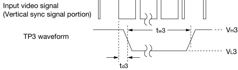
**\*8 V. SYNC switching voltage measurement**
