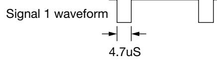
\*2 Measuring horizontal sync signal pull-in range for NTSC
