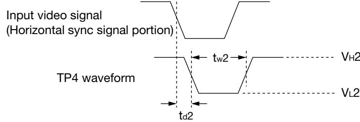
**\*7 V. SYNC measurement**
