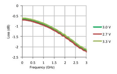
Figure 8. Active Port Return Loss vs V<sub>DD</sub> (RFX)
