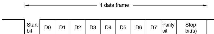
Figure 18-5. Asynchronous Serial Interface Transmit/Receive Data Format
