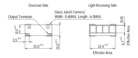
Note: Glass Substrate Thickness : 1.1mm Module Thickness : 1.3mm max Accepts normal soldering for bending.
