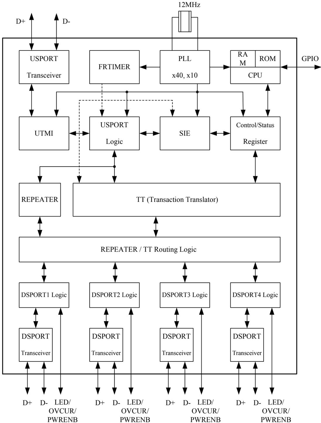
Figure 4.1 – GL850G Block Diagram (single TT)
