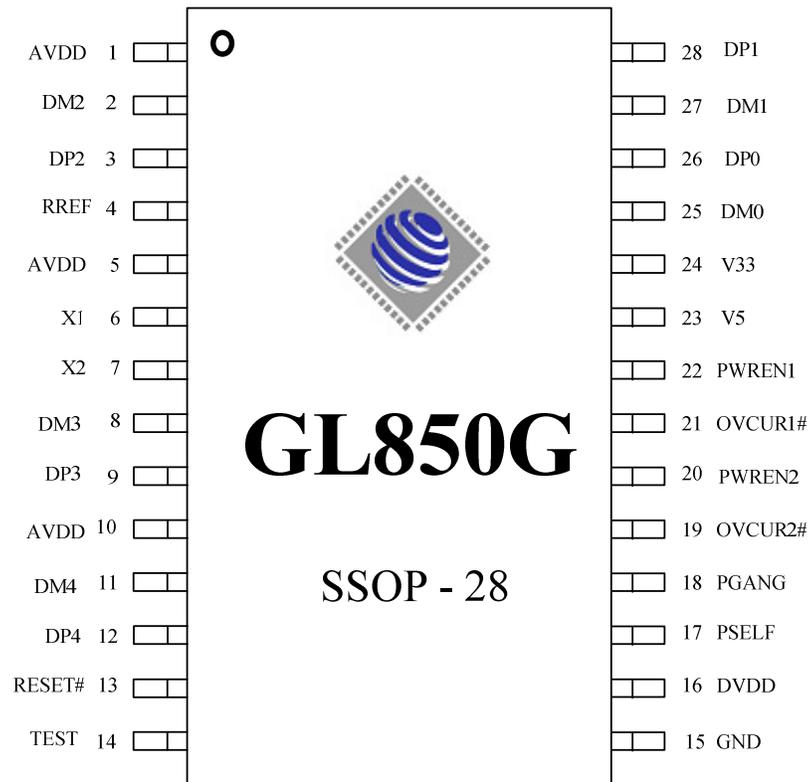
**Figure 3.2 – GL850G 28 Pin SSOP Pinout Diagram**
