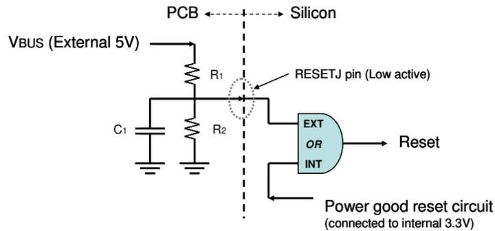
GL850G internally contains a power on reset circuit as depicted in the picture above
