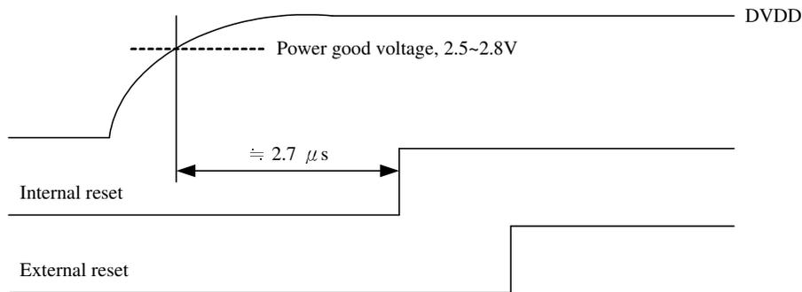
To fully control the reset process of GL850G, we suggest the reset time applied in the external reset circuit should longer than that of the internal reset circuit.
