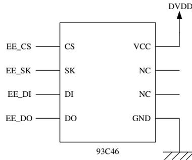
**Figure 5.9 – Schematics Between GL850G and 93C46**
