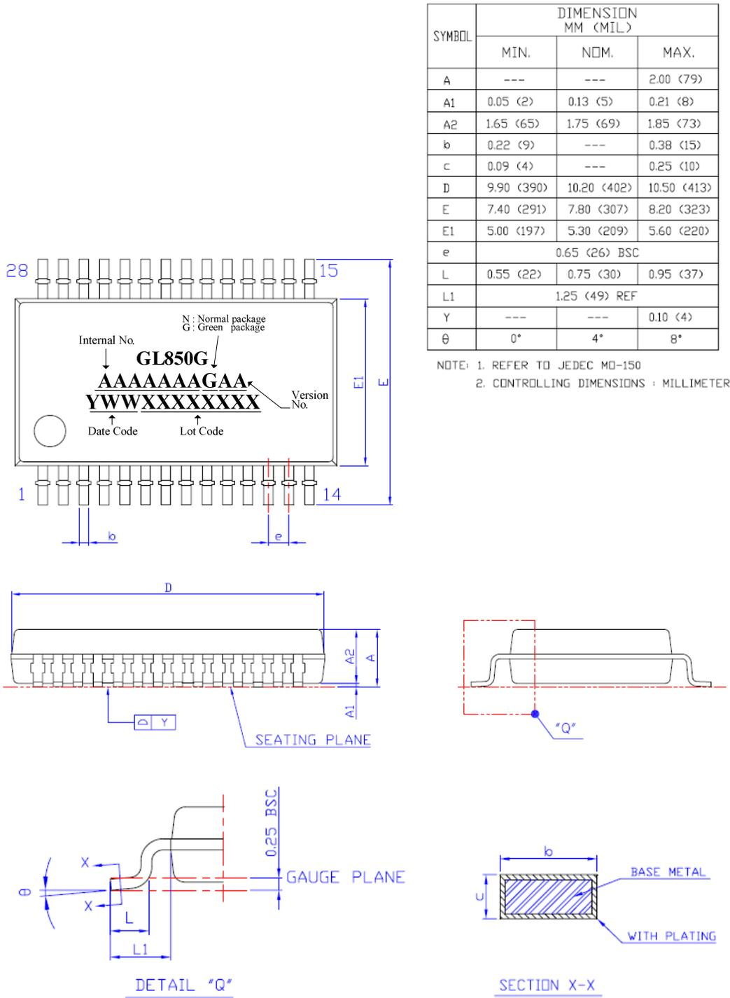
**Figure 7.2 – GL850G 28 Pin SSOP Package**
