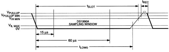
$\begin{array}{l} 60 \ \mu s \leq t_{LOW0} < t_{SLOT} < 120 \ \mu s \\ 1 \ \mu s \leq t_{REC} < \infty \end{array}$
