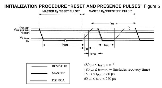
\* In order not to mask interrupt signaling by other devices on the 1-Wire bus,  $t_{RSTL} + t_R$  should always be less than 960 µs.
