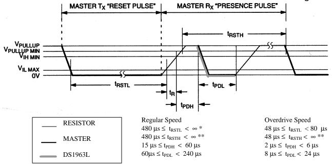
\*IN ORDER NOT TO MASK INTERRUPT SIGNALS BY OTHER DEVICES ON THE 1-WIRE BUS,  $t_{RSTL\ +\ tR}$  SHOULD ALWAYS BE LESS THAN 960  $\mu s$
