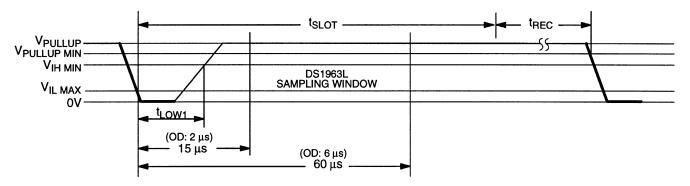
Regular Speed  $60~\mu s \leq t_{SLOT} < 120~\mu s$   $1\mu s \leq t_{LOW1} < 15~\mu s$   $1\mu s \leq t_{REC} < \infty$
