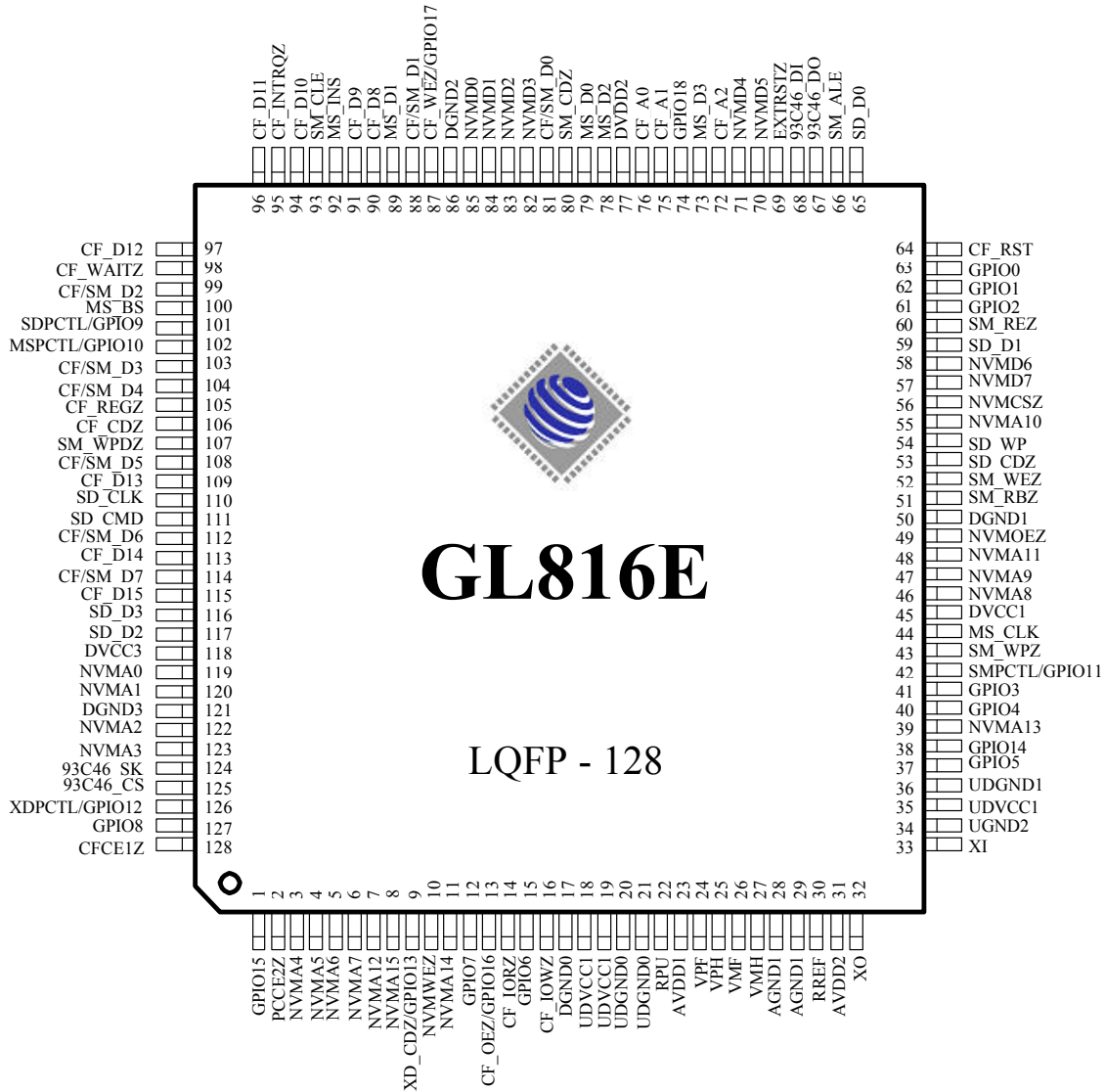
Figure 3.1 - 128 Pin LQFP Pinout Diagram
