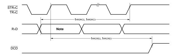
Note This bit is the MSB of BCS in the COP mode and MSB of the end flag in the BOP mode.
