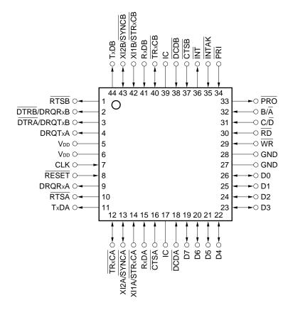
IC: Internally Connected (Leave this pin unconnected)
