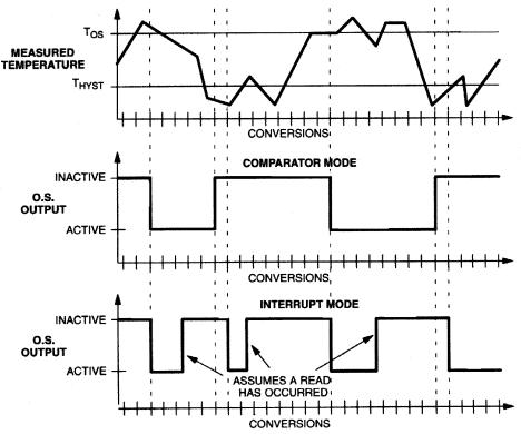
THIS TRANSFER FUNCTION ASSUMES THE DS75 IS CONFIGURED SUCH THAT 2 CONSECUTIVE CONVERSIONS OUT OF TOLERANCE CONSTITUTE AN O.S. FAULT.
