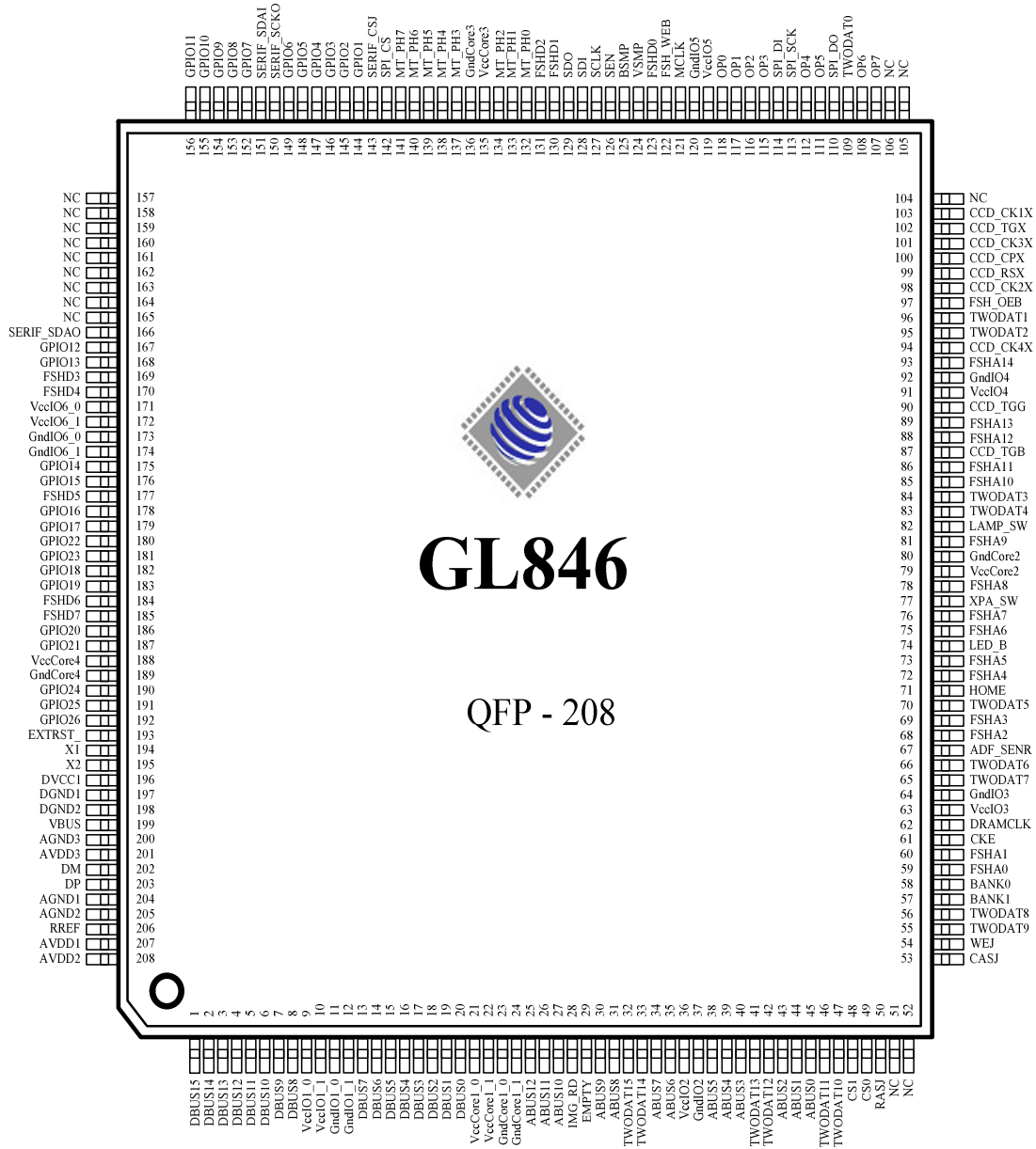
Figure 3.1 – 208 Pin QFP Pinout Diagram
