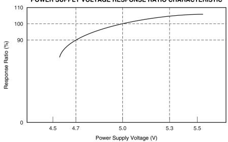
POWER SUPPLY VOLTAGE RESPONSE RATIO CHARACTERISTIC
