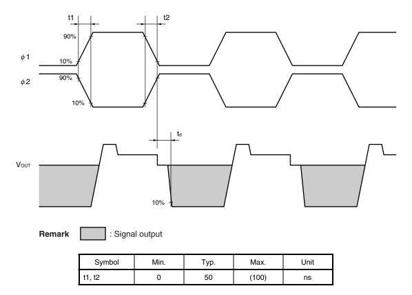
**Remark** The MAX. in the table above shows the operation range in which the output characteristics are kept almost enough for general purpose, does not show the limit above which the  $\mu$ PD3753 is destroyed.
