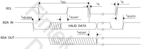
Serial Bus Timing Diagram
