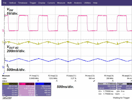
Steady State Operation V_{IN} = 5V, 39 \text{ LEDs}, 260mA
