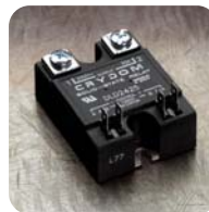
DSD, DLD Solid State Time Delay Control Relay 10-50Amp 120/240 Vac SCR AC Switch Output Externally Adjustable
