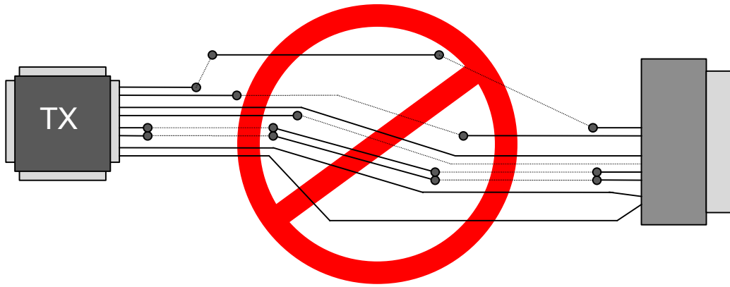
Figure 19. Example of Incorrect Differential Signal Routing
