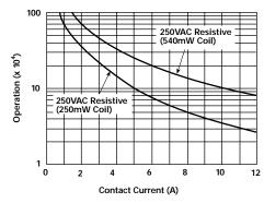
Note: This data is based on the max. allowable temperature for E type insulation coil (115°C).
