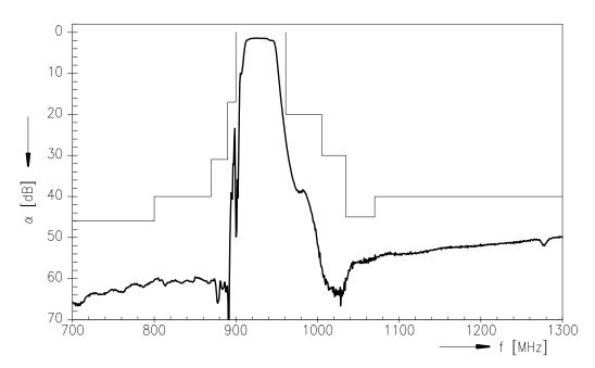
Transfer function (pass band, 25  $\pm$  10  $^{\circ}\text{C})$
