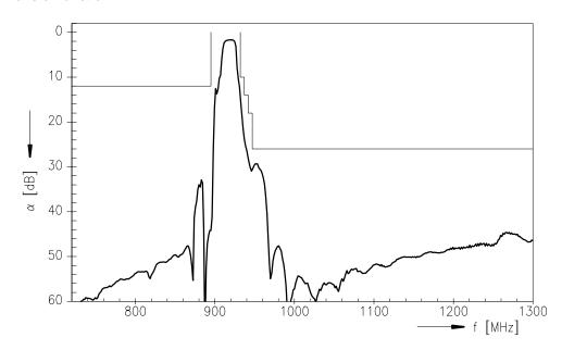
Transfer function (pass band, 25  $\pm$  10  $^\circ\text{C})$
