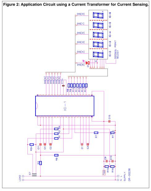
Note: Capacitor C11 may be selected for phase compensation and DC blocking.
