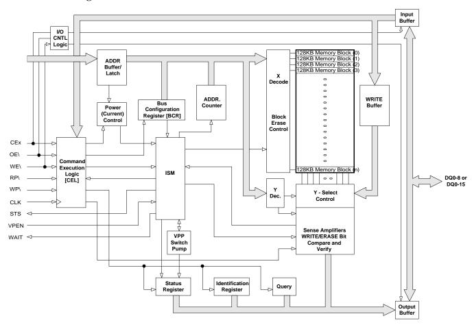
Additionally, the Scaleable Command Set [SCS] allows a single, simple software driver in all host systems to work with all SCS compliant FLASH memory devices. The SCS provides the fastest system/device data transfer rates and minimizes the device and system-level implementation costs.
