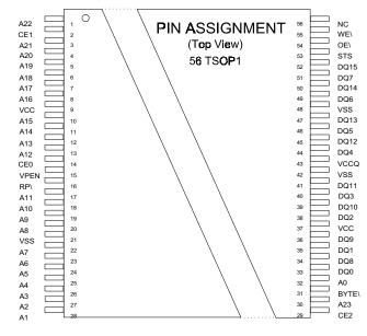
This device features in-system block locking. They also have a Common FLASH Interface [CFI] that permits software algorithms to be used for entire families of devices. The software is device-independent, JEDEC ID-independent with forward and backward compatibility.
