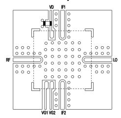
**App Note [1] Biasing** - Please refer to the functional block diagram and pin-out table for biasing information. The device is operated by biasing VD=4.0V with ID=180 mA by adjusting the applied voltage on VG1.VG1 typically requires-0.5V to result in the drain current being 180mA. The nominal input impedance of this gate is 1800hm, so it should be noted that the nominal gate current will be 2.7mA.
