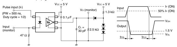
$\ensuremath{\text{CL}}$  includes probe and stray wiring capacitance.
