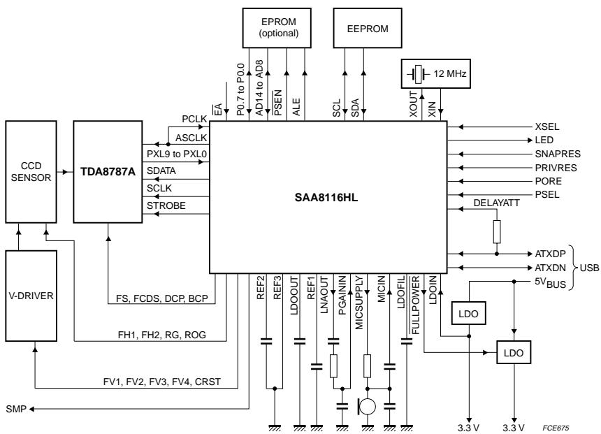
Digital PC-camera signal processor,
