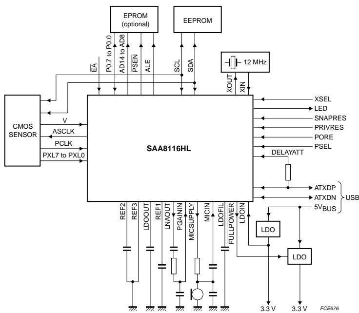
Fig.4 CMOS sensor application.
