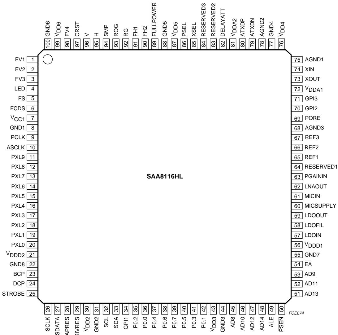
Fig.2 Pin configuration.
