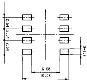
Please apply resist processing to the area around the electrode pads.
