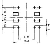
Please apply resist processing to the area around the electrode pads.
