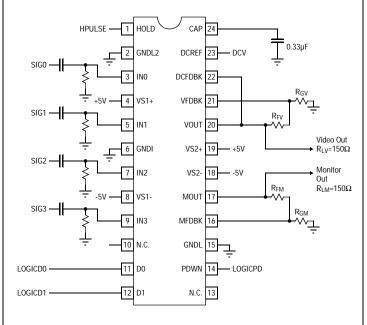
Note: Pin #6 should be a good high frequency ground
