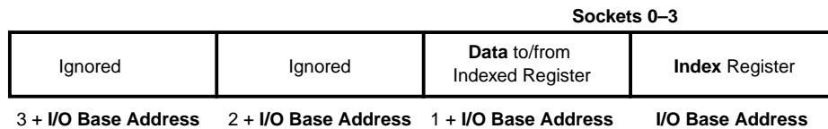
Figure 7-1. Operation Registers as PCI Doubleword I/O Space at I/O Base Address Register (Programmed at Configuration Space, Offset 44h)
