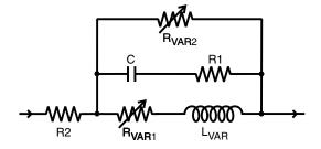
The value of the frequency-dependent variable resistor  $\mathsf{R}_{VAR1}$  is calculated from:
