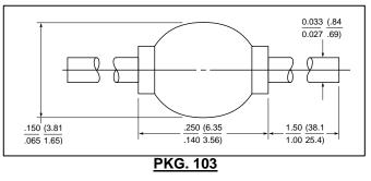
Note: The cathode side is marked with a dark colored band on the diode body.
