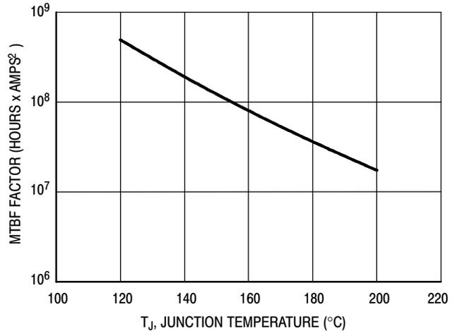
This above graph displays calculated MTBF in hours x ampere<sup>2</sup> drain current. Life tests at elevated temperatures have correlated to better than  $\pm 10\%$  of the theoretical prediction for metal failure. Divide MTBF factor by  $I_D^2$  for MTBF in a particular application.
