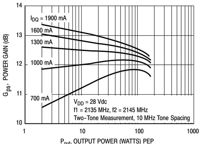
Figure 4. Two-Tone Power Gain versus Output Power
