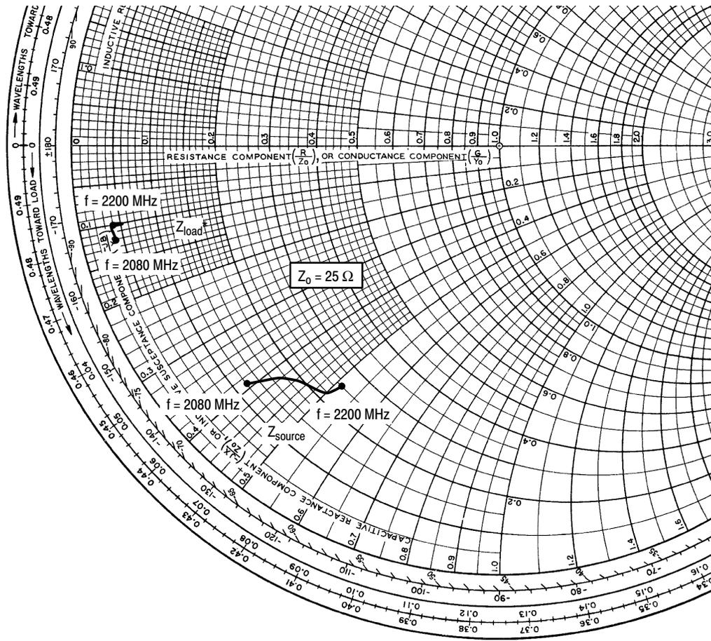
$V_{DD} = 28 \text{ Vdc}$ ,  $I_{DQ} = 1300 \text{ mA}$ ,  $P_{out} = 33 \text{ W Avg.}$
