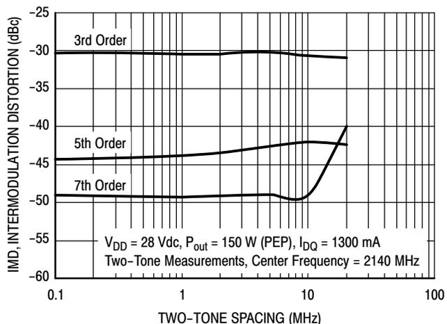
Figure 6. Intermodulation Distortion Products versus Tone Spacing
