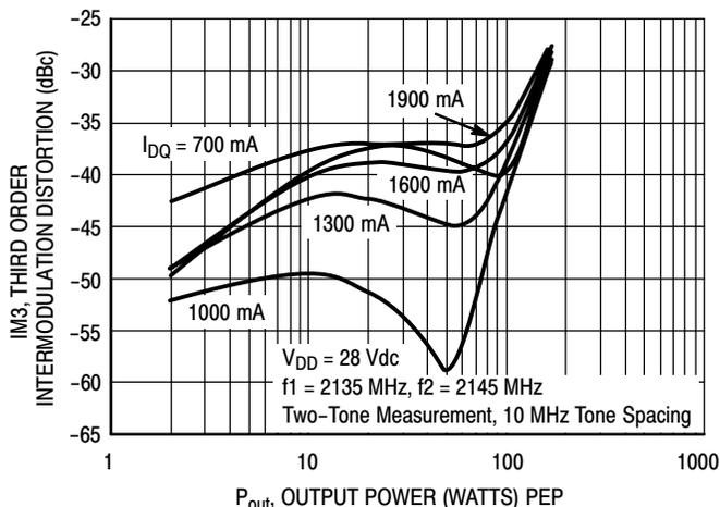
Figure 5. Third Order Intermodulation Distortion versus Output Power
