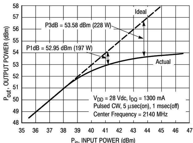
Figure 7. Pulse CW Output Power versus Input Power
