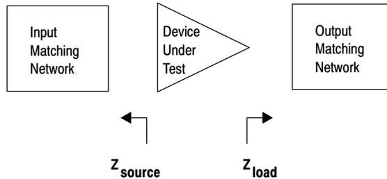
Figure 12. Series Equivalent Input and Output Impedance
