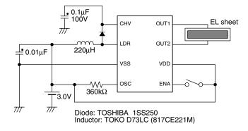
Note: Do not operate the SM8144B with the EL sheet NOT connected (no load to OUT1/OUT2) since the IC will be damaged.
